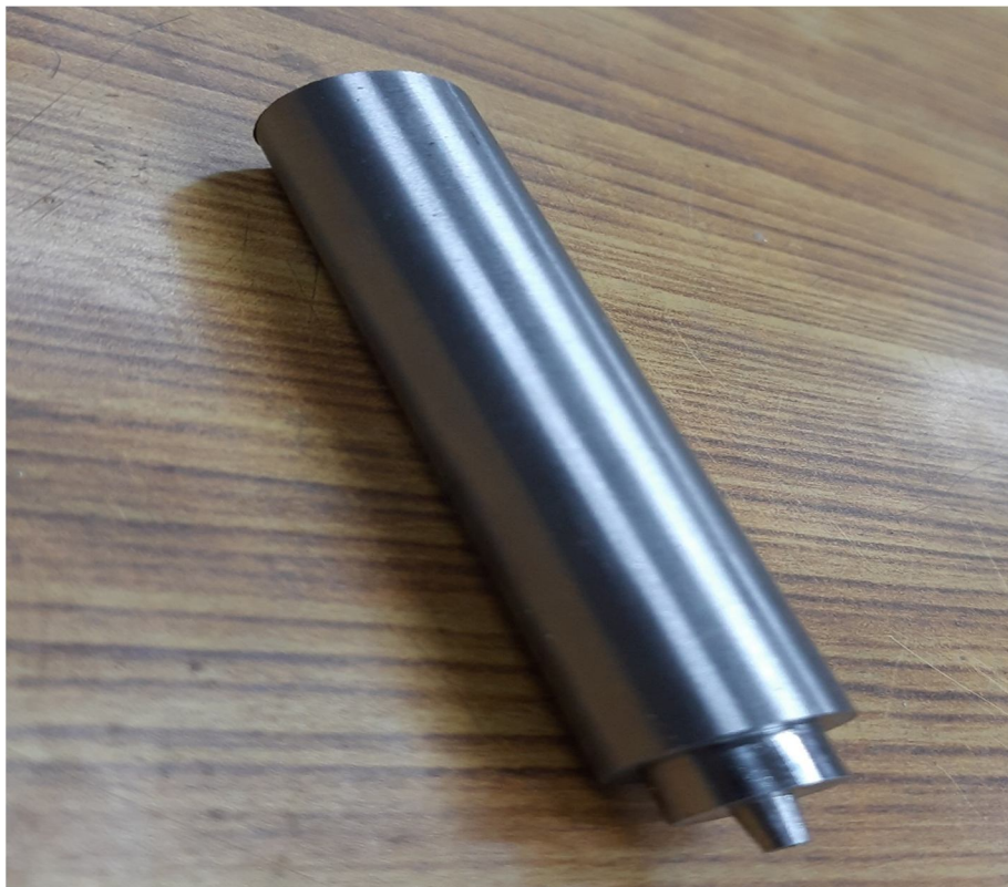
Figure 7. FSW Tool (14mm )
