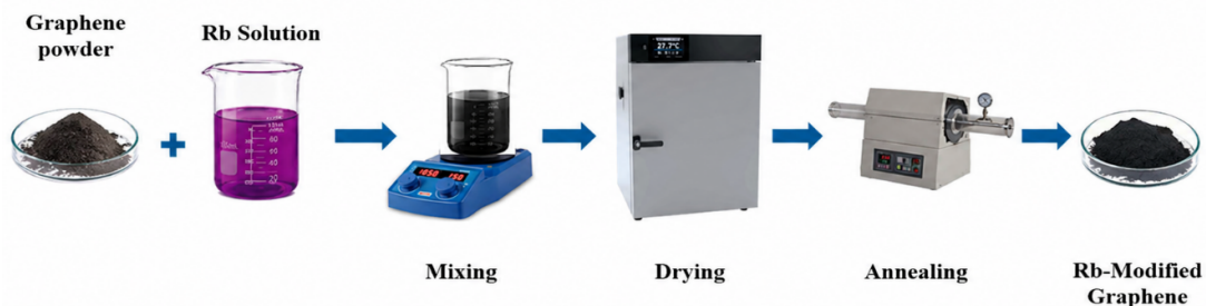
Fig 1: Stepwise Synthesis of Rb Modified Graphene
