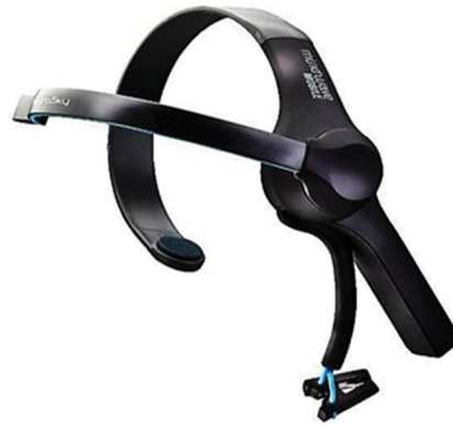
Fig. 2 Neurosky MindWave Single-Channel EEG Headset
