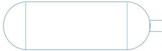
Figure 1. Type-1 CNG Cylinder (All Metal)
