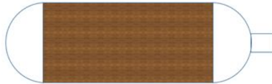
Figure 2. Type-2 (Metal body + Reinforced hoop wrap only)
