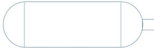
Figure 1. Type-1 CNG Cylinder (All Metal)
