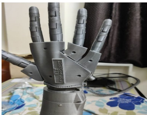
Fig 7: - gesture replicating robot arm
