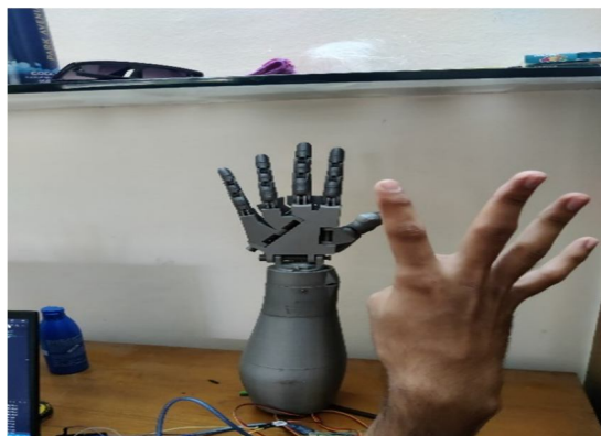
Fig 12: - Shows Testing of hand (4 finger as input)
