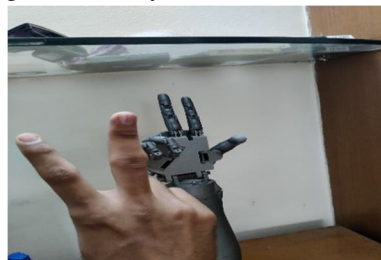
Fig 11: - Shows Testing of hand (2 fingers as input)
