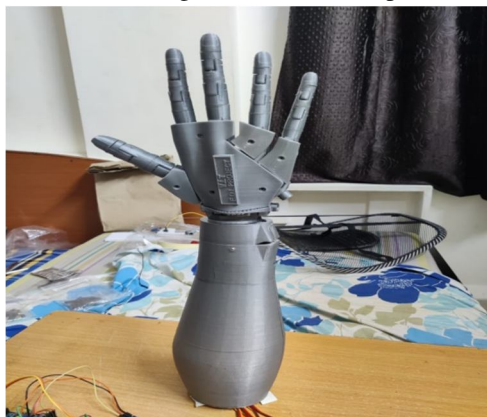
Fig 3: - 3d printed Robo Arm
