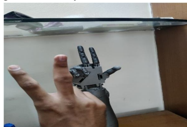
Fig 11: - Shows Testing of hand (2 fingers as input)
