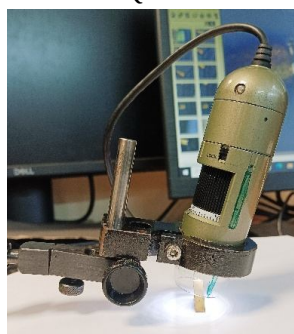
Dinolite digital microscope for tool wear measurement
