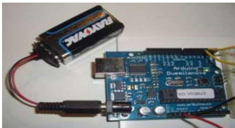
Fig. 2.3 Arduino microcontroller hardware
