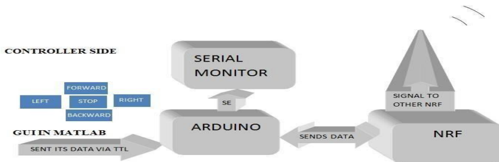
Fig. 3.1 Controller side block diagram
