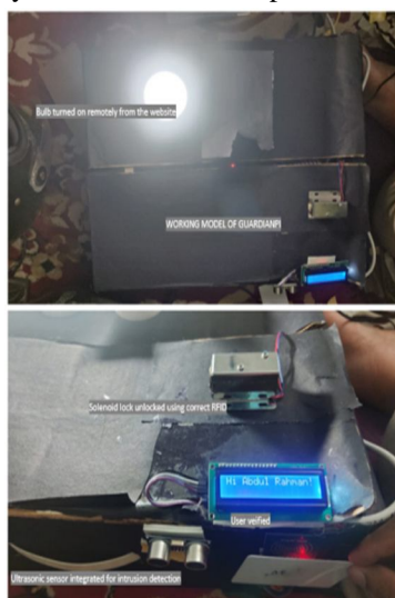
Fig. 12 Physical Model of the GuardianPi System
