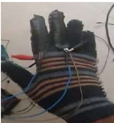
Fig.5. The system produces “Hello, Good morning” while using this hand gesture to communicate.
