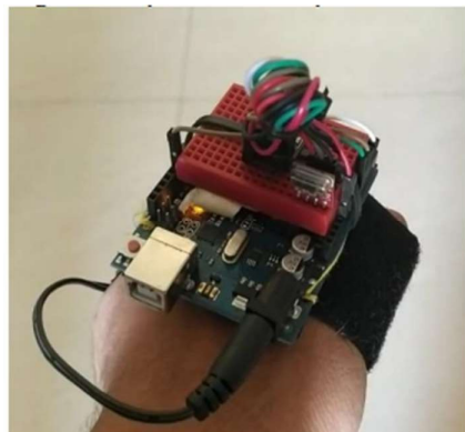
Figure 8 Implemented prototype Hand Gesture control gloves
