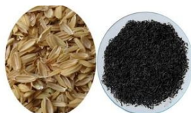
Fig 1. Rice husk Before and After Filtration
