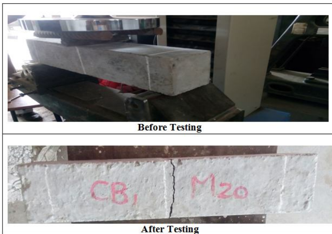
Fig. 10 Beam flexural test
