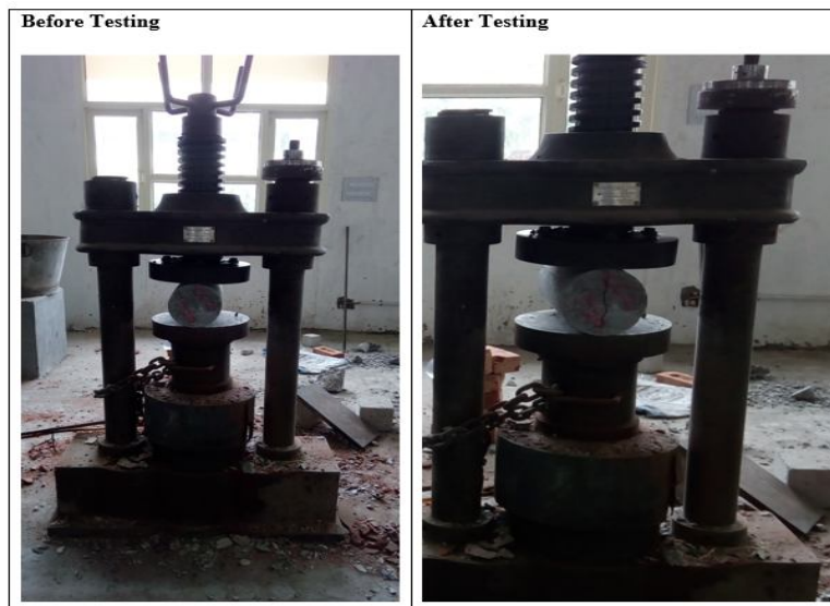
Fig.7 Cylinder Split Tensile Strength
