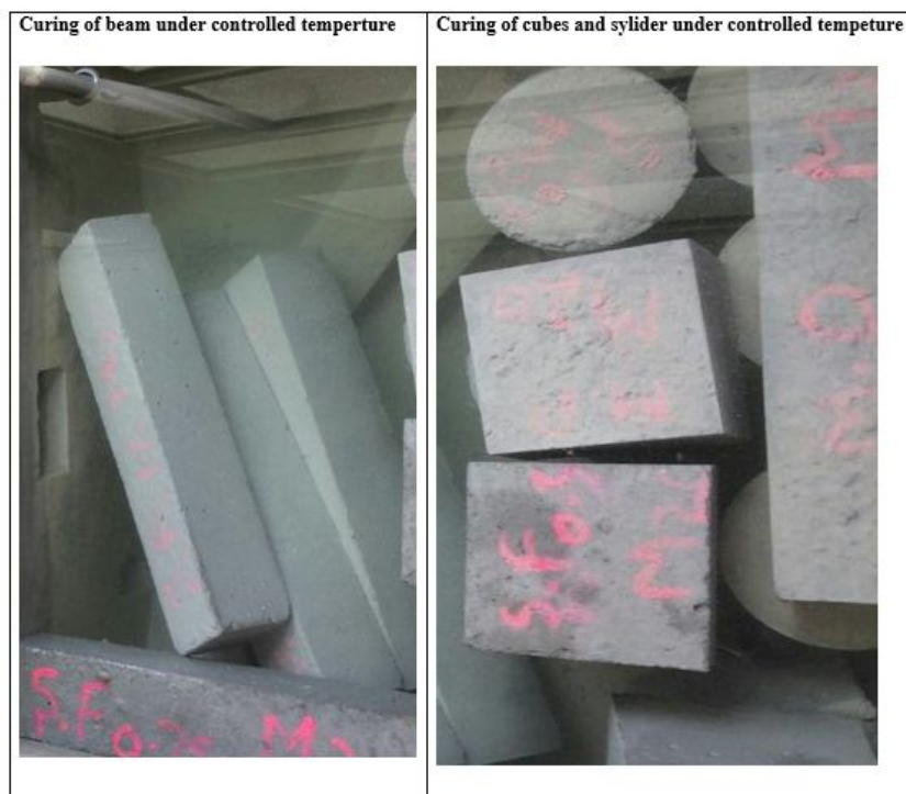
Fig.5 Specimen is placed in a curing tank.
