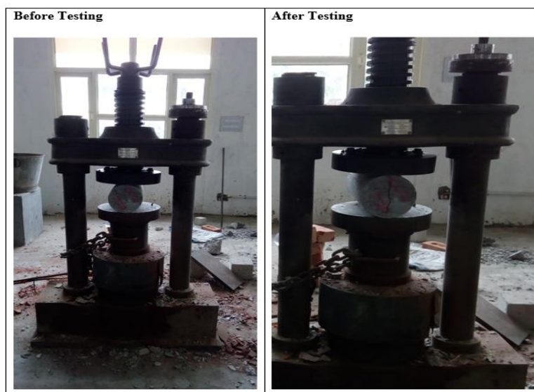
Fig.7 Cylinder Split Tensile Strength
