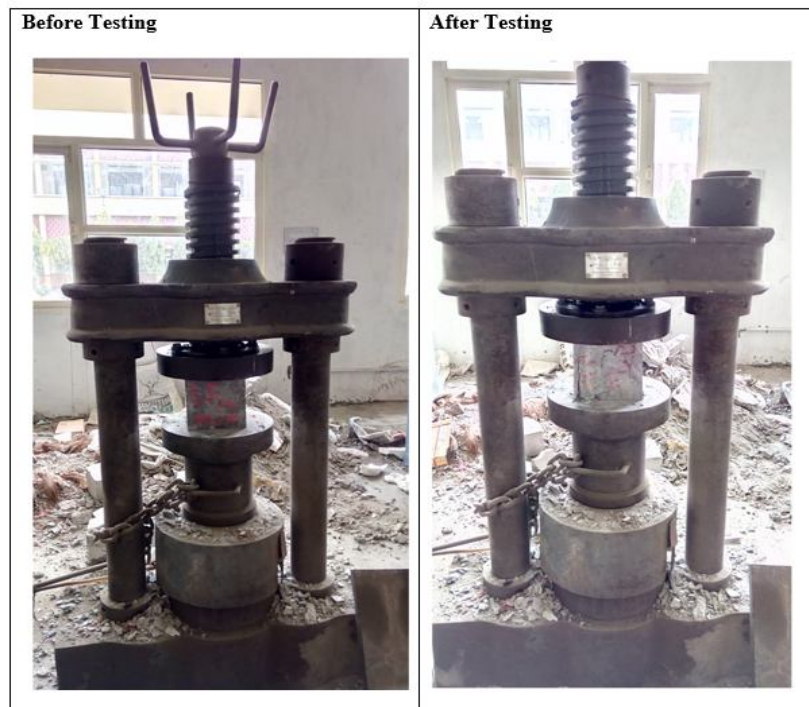
Fig.6 Compression Cube Test
