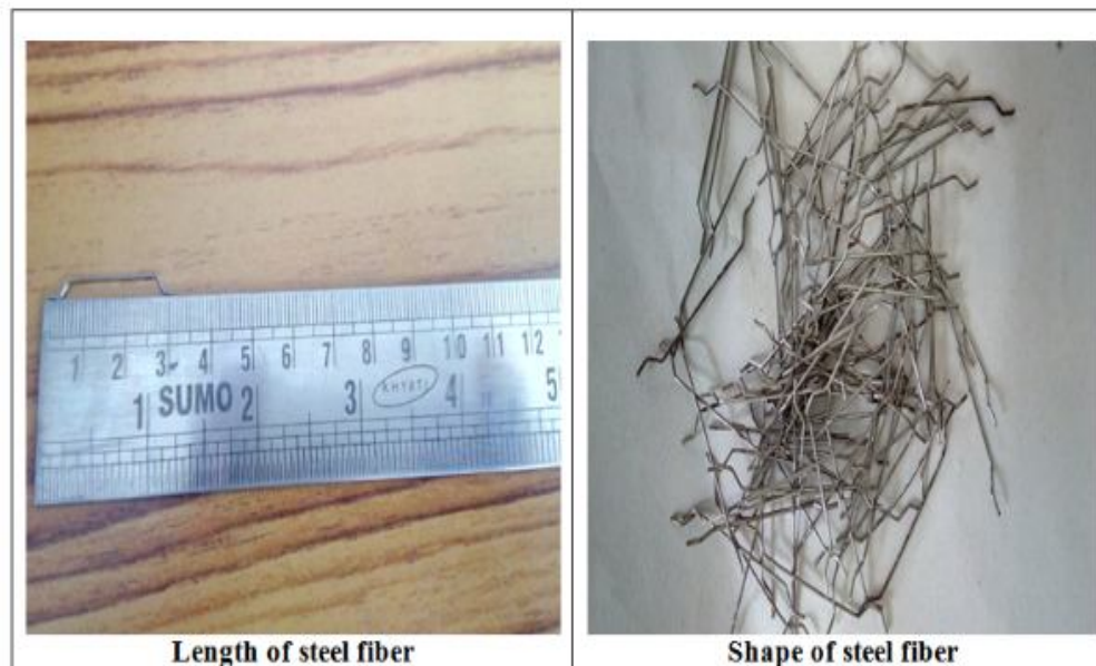
Fig.2 Hooked End steel fibers
