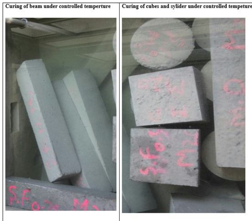
Fig.5 Specimen is placed in a curing tank.
