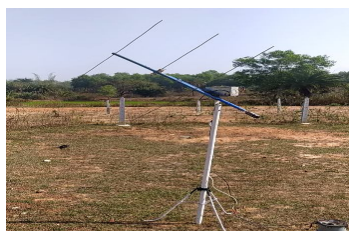
Fig. 11- Testing Rotator with Associated load
