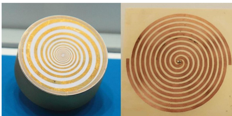
Figure 4. Two-arm, tightly-wrapped, logarithmic and Archimedean spiral antennas
