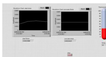
Fig 5.2 Strain corresponding to 500kg(5KN/M) while unloading
