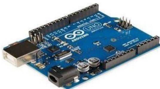
Fig.1 Arduino Board(A Tmega 328P Microcontroller)
