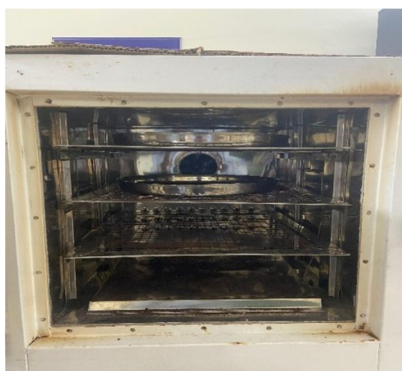
Fig 2.1.4 Baking at 145°C for 45 min
