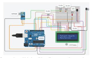
This is the TinkerCad circuit diagram of our project which describing all sensors and connections.
