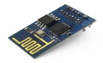
This is a ESP8266 Wi-Fi module which sends measured data to the ThingSpeak IoT sever.
