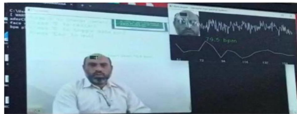
Fig 4(b): Displaying the heart rate through the input face image as 79.5 bpm.
