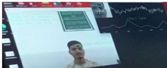
Fig 4(c): Displaying the heart rate through the input face image as 100.1 bpm.
