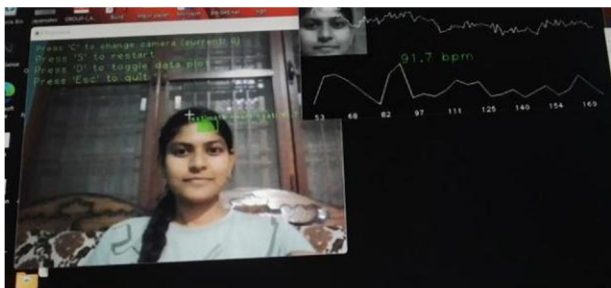
Fig 4(a): Displaying the heart rate through the input face image as 91.7 bpm.
