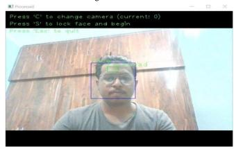
This face recognition algorithm is applied to the frame in the video and outputs a bounding box for each face it detects. To maintain consistency across frames, if there is no face detected in frame ,the face from the previous frame is used, if there is multiple face detected in the frame, the face that is nearest to that frame is used.
