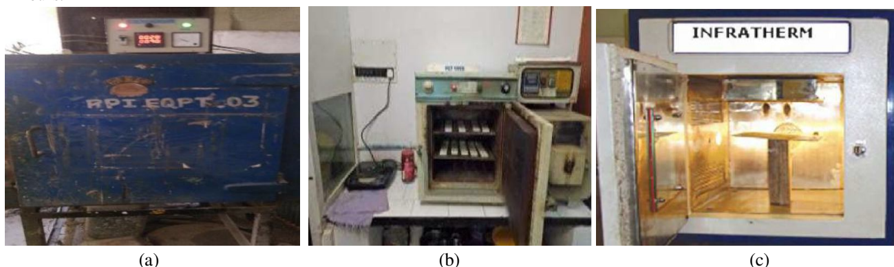
Fig-2: (a) Conventional hot air heating, (b) Microwave heating and (c) Infrared heating
