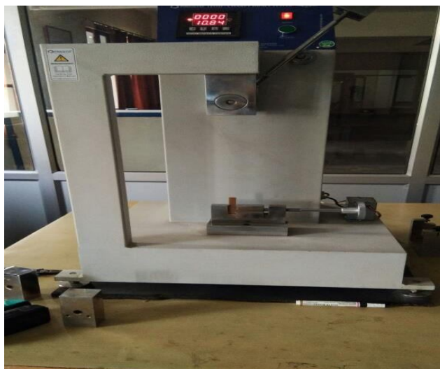
Fig. 2.1.2 Impact testing machine with Sample loaded condition
