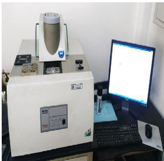
Fig. 2.2.1 LFA 447 used for thermal conductivity, thermal diffusivity and bulk density
