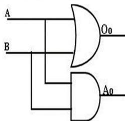
Figure 7 Logic diagram of AND-OR gate block
