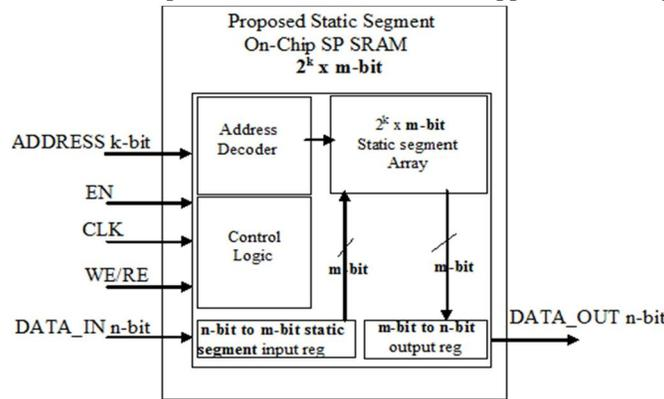
Figure 8 Architecture of proposed m-bit SSOC SP SRAM
