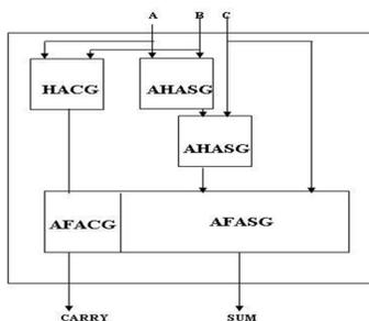
Figure 2 Simplified block diagram of proposed AFAL2
