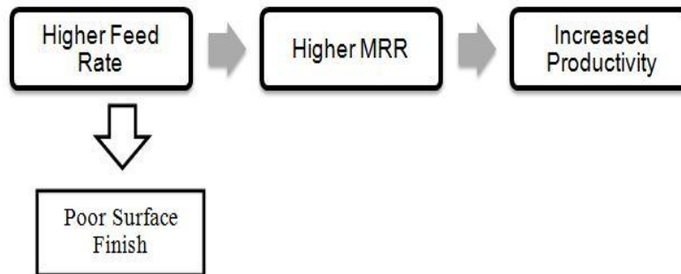
Fig (e) Effect of Feed rate on surface roughness
