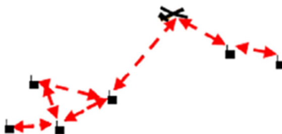
Fig. 1 Using UAV to relay between ground stations [1]
