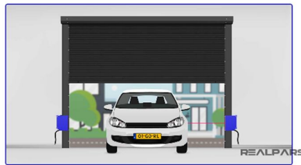
Fig. 4 Photoelectric Beam Sensor. Source: [3]
