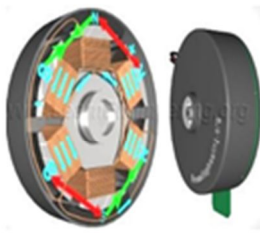
Fig. 3 Internal structure of BLDC motor
