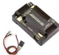
Fig. 6 APM Controller Board
