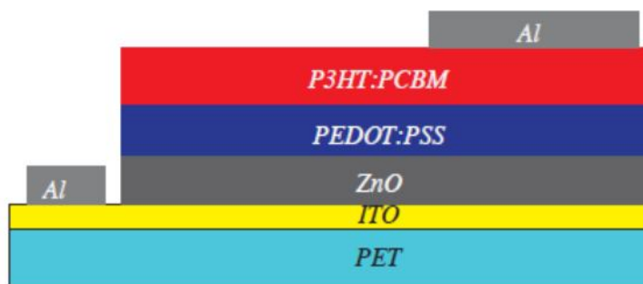
Figure 1. Schematic representation of the hybrid solar cell
