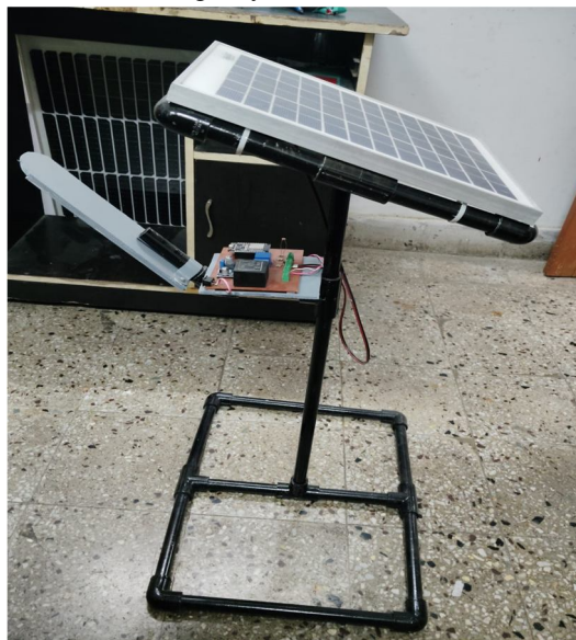
Figure 4.2: Overall View of the Prototype Hybrid Solar Street-Light Model
