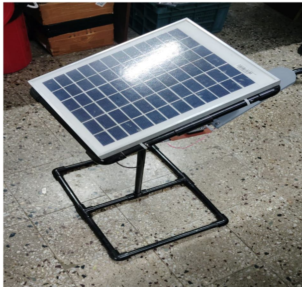
Figure 4.1: Top View of Solar Photovoltaic Panel Mounted on the Prototype
