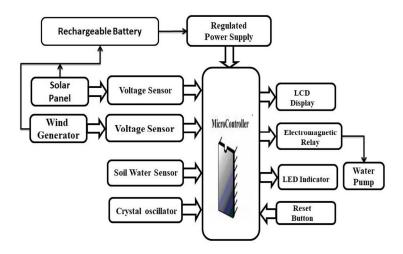
Fig: block diagram of hybrid water pumping control system for irrigation by using ardunio
