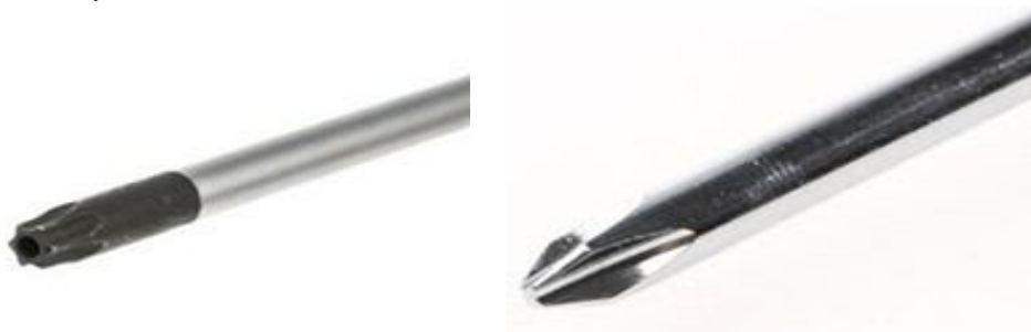
Fig. 3: Torx Key and Phillip Key Comparison
