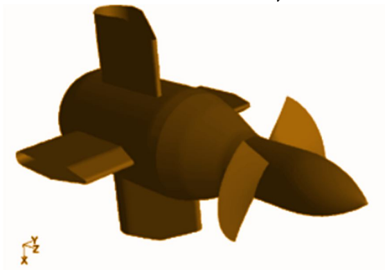
Fig.14 Swirl type turbine model [37]
