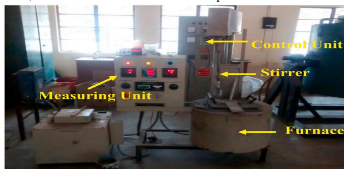
Fig. 2. Stir casting process setup.
