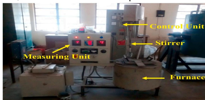
Fig. 2. Stir casting process setup.
