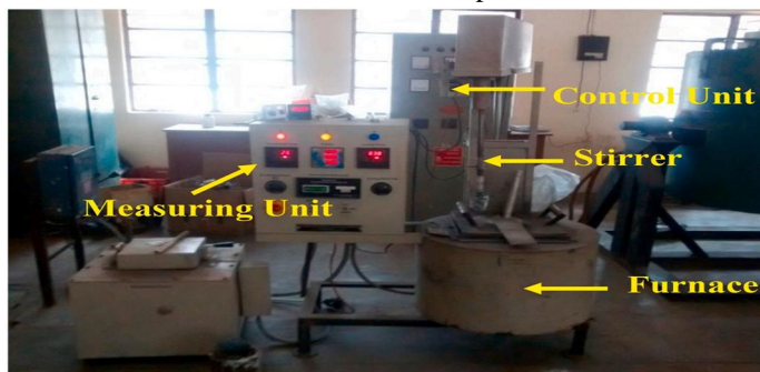
Fig. 2. Stir casting process setup.
