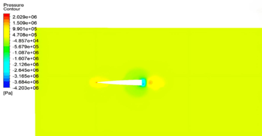
Figure 38. Pressure Contour of LD-Haack Series Nose Cone at Mach 12
