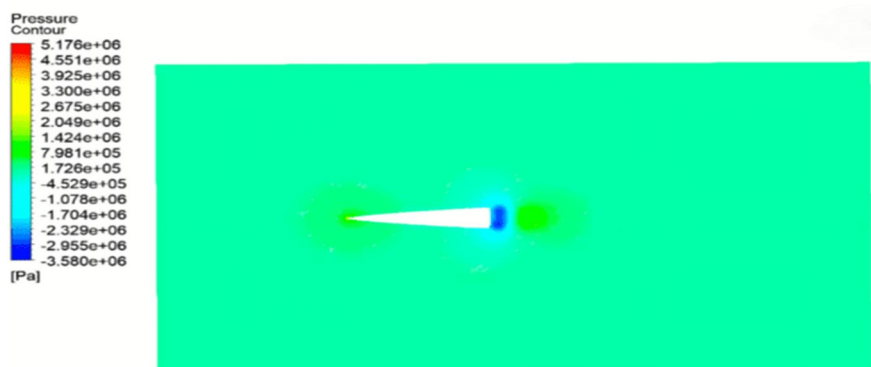
Figure 53. Pressure Contour of Power Series Nose Cone at Mach 11
