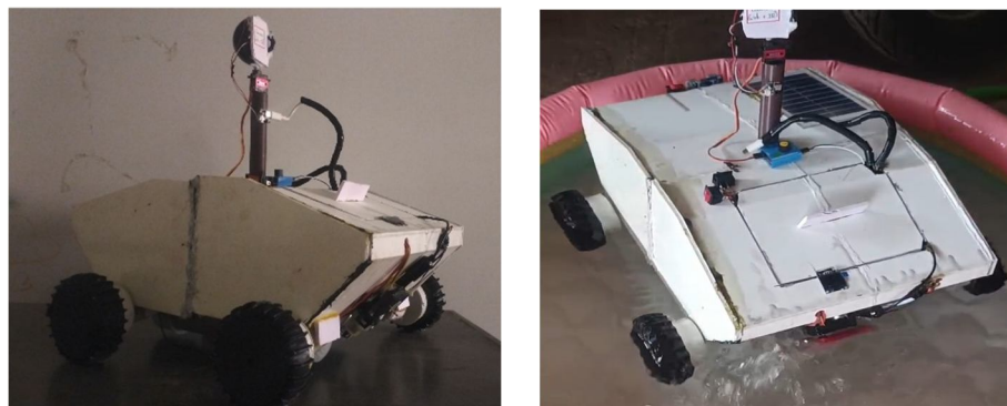
Fig. 3 Physical Model of Amphibious Robot on Land and Water
