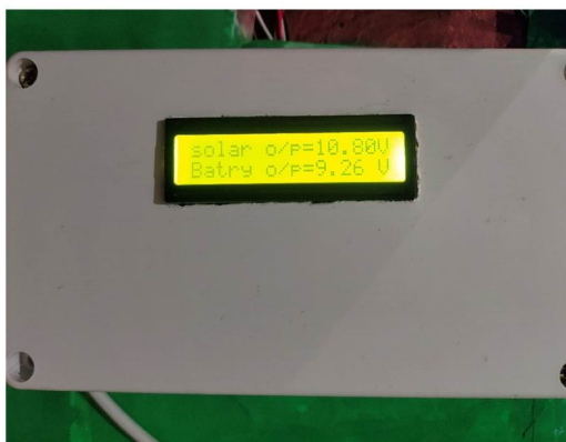
Fig. 7: Home battery starts charging when Home battery < 12V AND Solar Output > 10V
