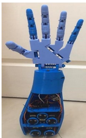
Figure 6: 3-D printed Prosthetic Hand
