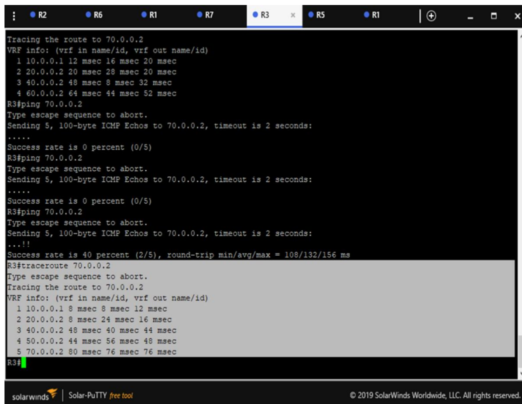
Fig.4 Result of BGP choosing the best path which is not busy when no path is busy
