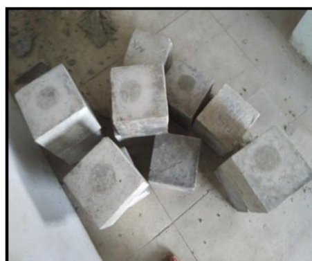
Figure 4.4: Cubes After Completion Of Curing Period
