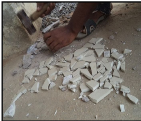
Figure 3.9: Manual Crushing Of Waste Tiles
