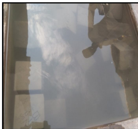
Figure 4.3 Curing Of Cube Specimen
