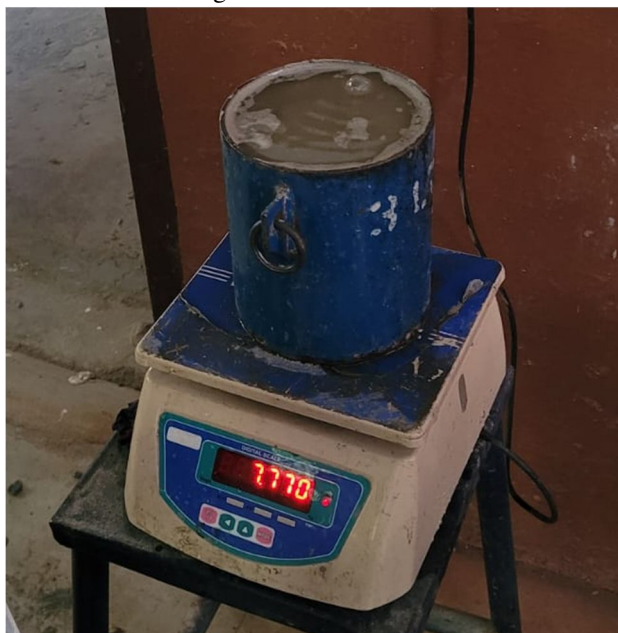
Fig 7: Specific gravity test for Fine aggregate
