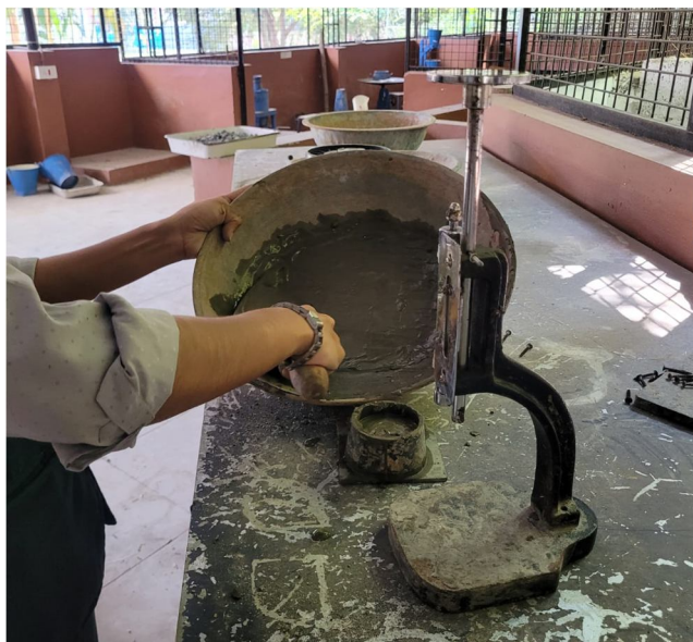
Fig 4: Standard consistency test using Vicat's apparatus
