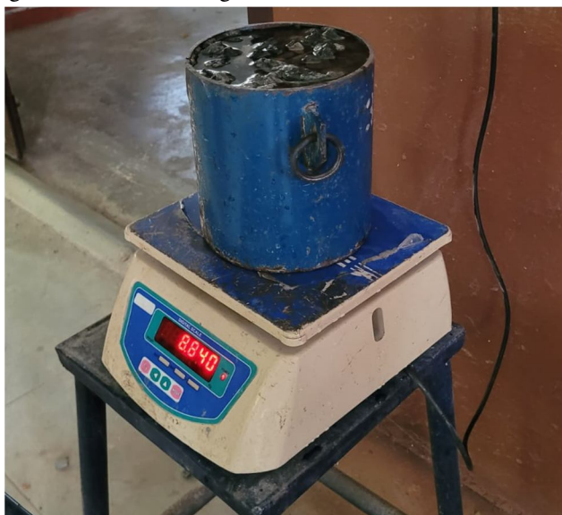
Fig 8: Specific gravity test for Coarse aggregate
