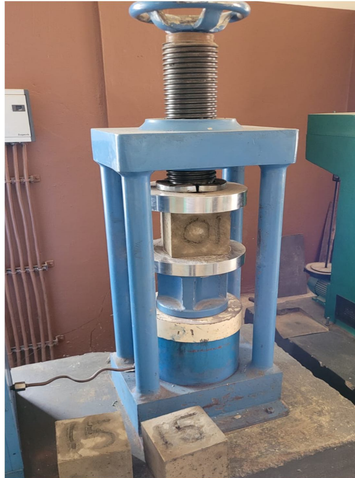
Fig 12: Compressive strength test on CTM
