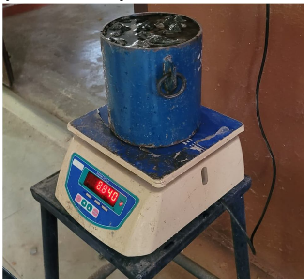
Fig 8: Specific gravity test for Coarse aggregate
