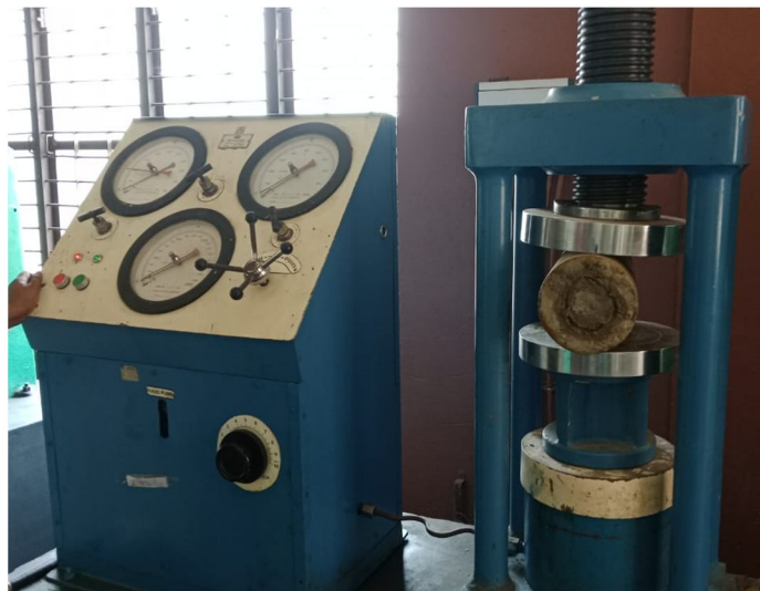
Fig 15: Split tensile strength test on CTM
