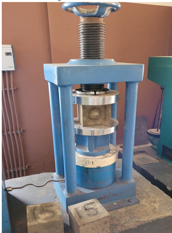
Fig 12: Compressive strength test on CTM
