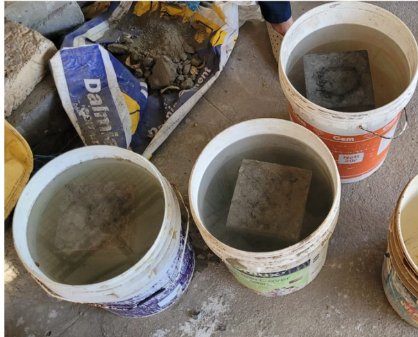
Fig 16: Test specimens kept for curing in 5% H 2 SO 4
