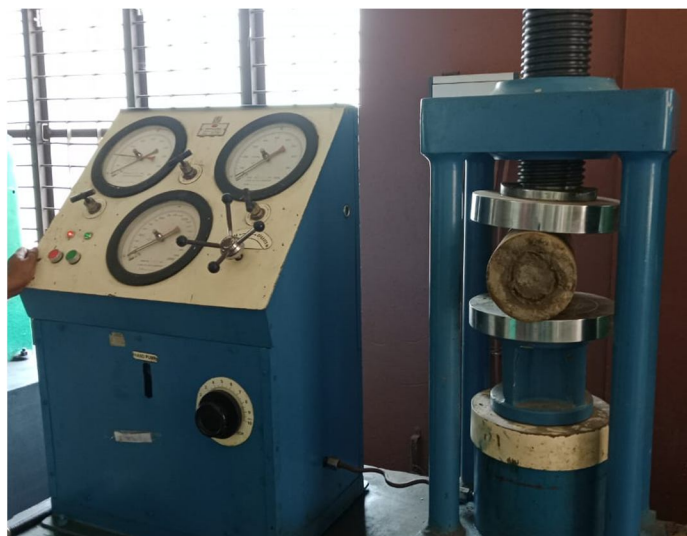
Fig 15: Split tensile strength test on CTM
