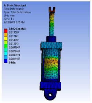
Above figure shows total deformation in the hydraulic jack.
