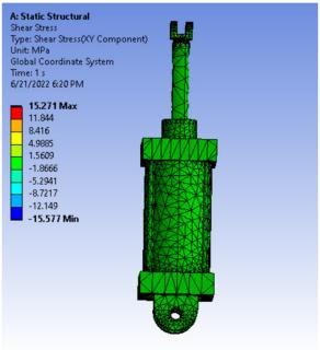
Above figure shows shear stress in the hydraulic jack.
