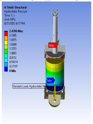
This figure shows us internal tank pressure due to hydraulic oil i.e. 1.6264 MPa (yellow part) and theoretically we got 1.31 MPa. This verifies that our hydraulic jack is feasible and we can use it for our purpose. Following are some results of the simulation.
