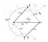
From the procedure, the fundamental cut-sets of the above graph are,
