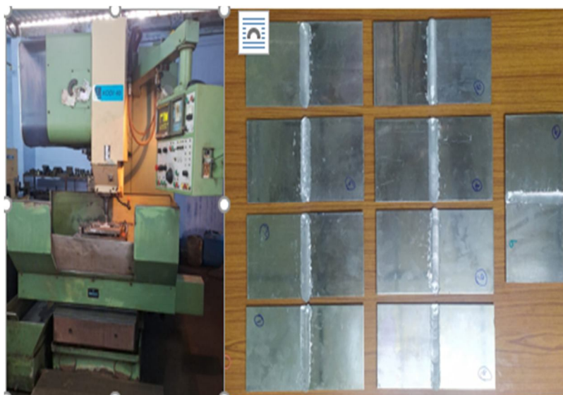
Fig. 3 VMC Setup & FSW trials from different tool profiles
