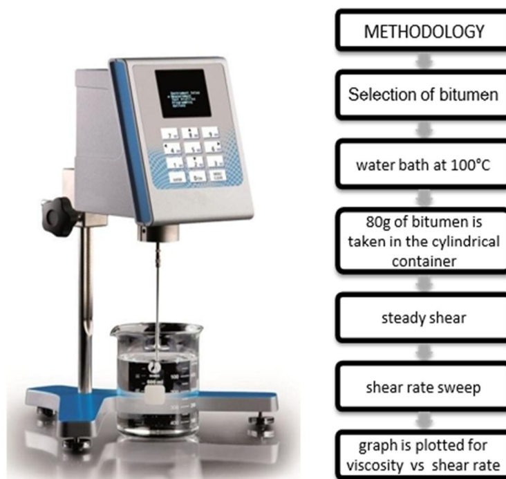
Fig 1: Viscometer and its methodology
