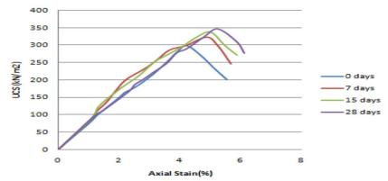
The below graph shows the UCS value of optimum mix of cement with different curing period. It has been observed that as the number of curing days increases the UCS value is also increases and at the end of 28 days the UCS value is 1995.56kN/m<sup>2</sup>. The UCS value is more as compared to optimum mix of steel slag.
