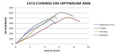
From Graph, it has been clearly observed that there is a gain in the strength values for the samples treated with optimum mix proportion. This increase in value can be explained by the fact that steel slags contain certain minerals that contribute to the pozzolanic reaction that contributes to the formation of a compound which leads to strength of the mix.
