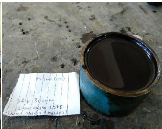
Figure 4.2:-Sample for Penetration Test
