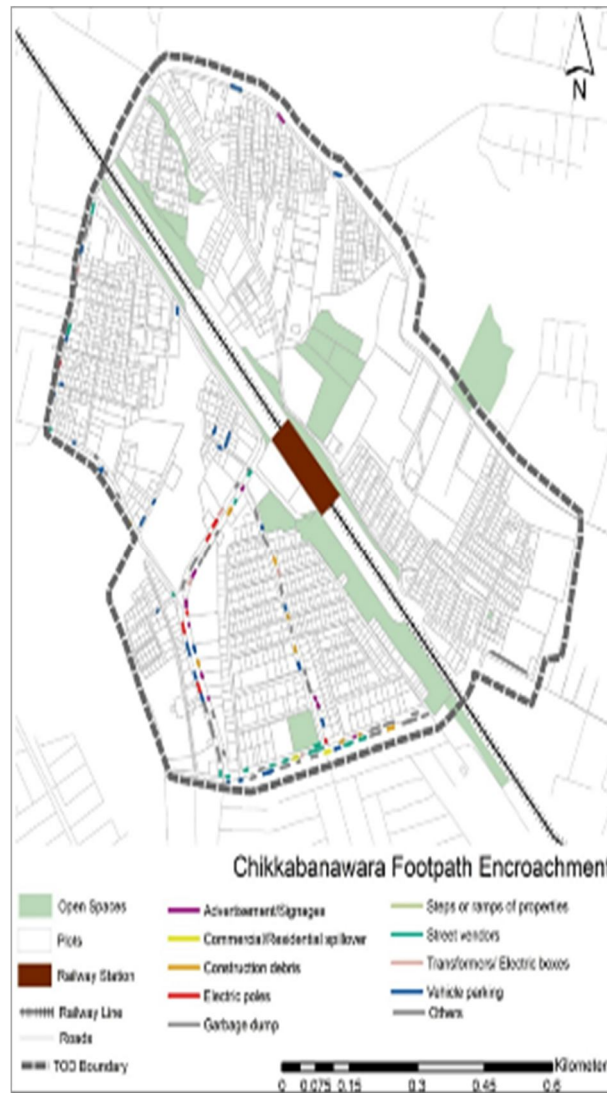
Figure 17: Chikkabanawara Footpath Encroachment map Source: Author
