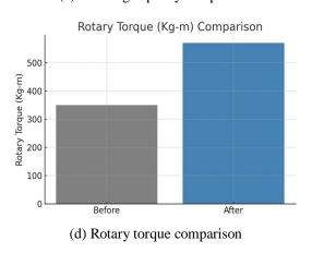
Figure 1. Comparison of key performance parameters before and after rig rehabilitation: (a) Service life, (b) Hoisting capacity, (c)
