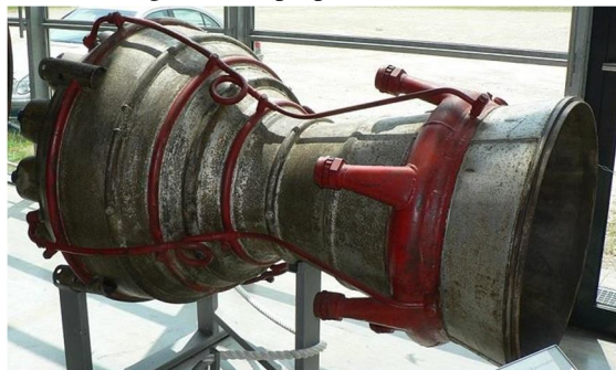
Figure 4.4: Convergent-divergent nozzle design: CD Nozzle
