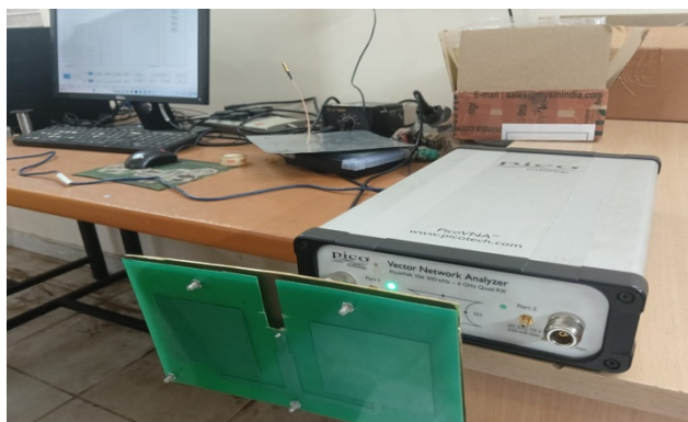
Figure 6 Taking Readings Of antennas Using Vector Network Analyzer (VNA)
